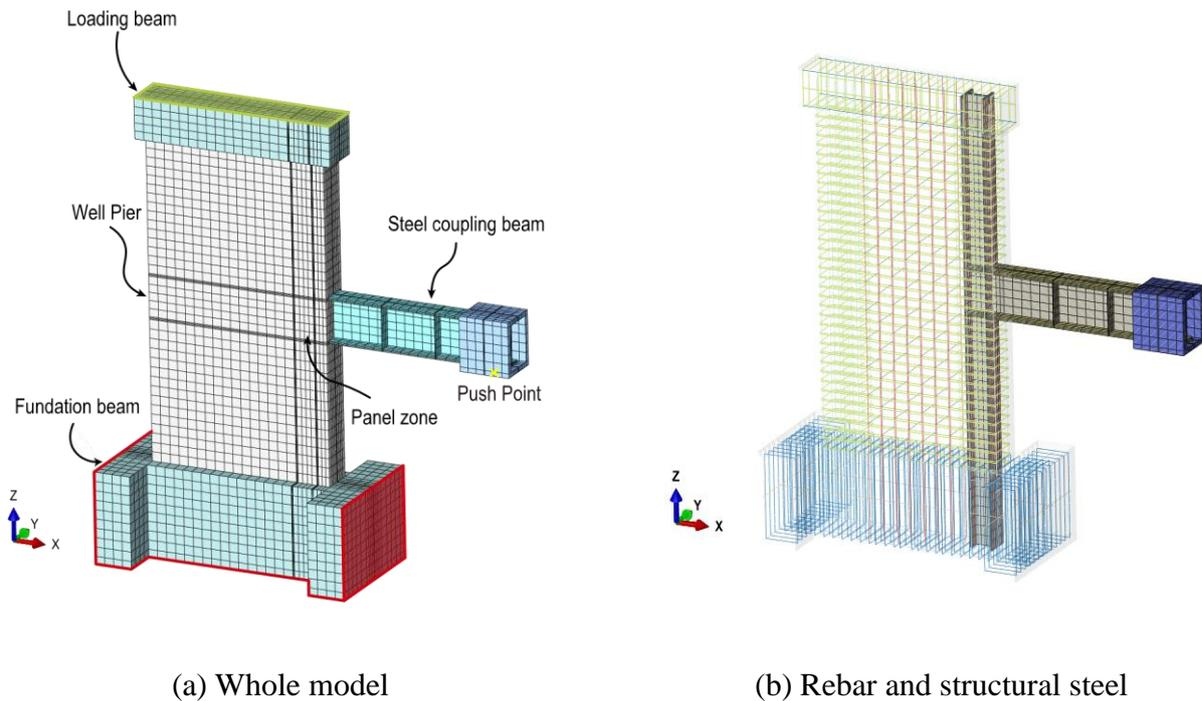
**Fig. 10.** Finite element model of specimen.
