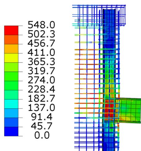
(b) Equivalent plastic strain of reinforcement
