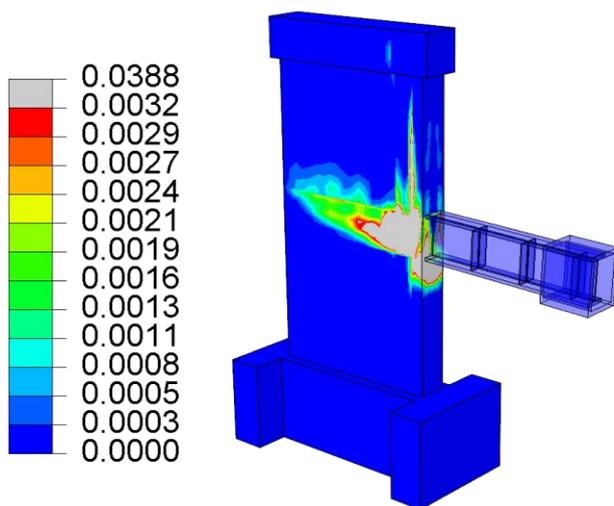
(a) Equivalent plastic strain of concrete
