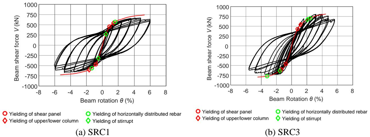
**Fig. 11.** Analytical curves of shear load versus beam rotation for specimens.
