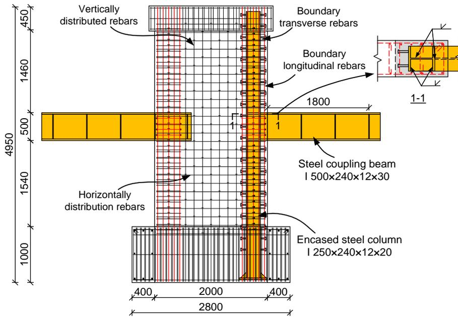
(b) Elevation drawing of steel reinforcement for SRC1
