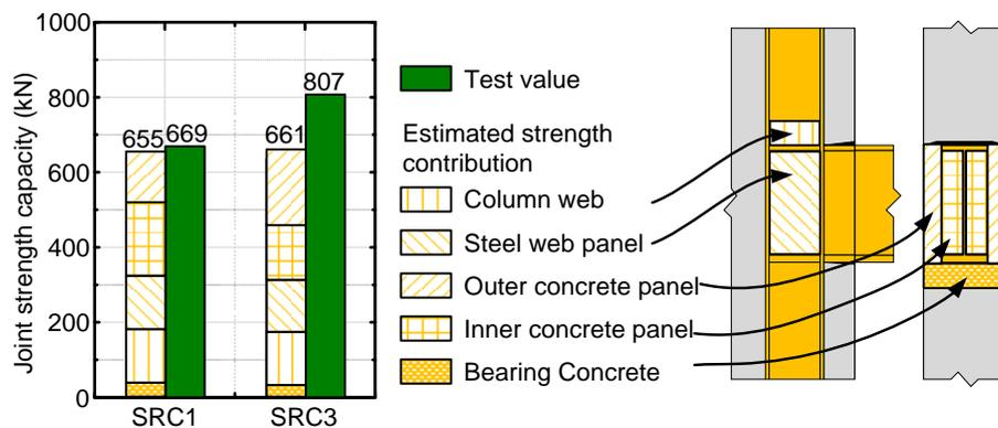
**Fig. 9.** Estimated strength capacity for specimens.
