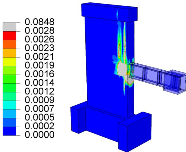
(a) Equivalent plastic strain of concrete
