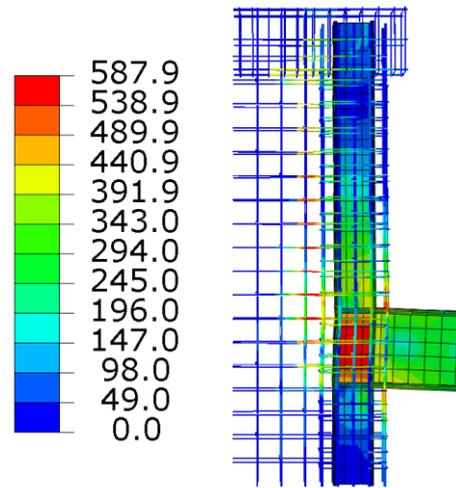
(b) Equivalent plastic strain of reinforcement and structural steel
