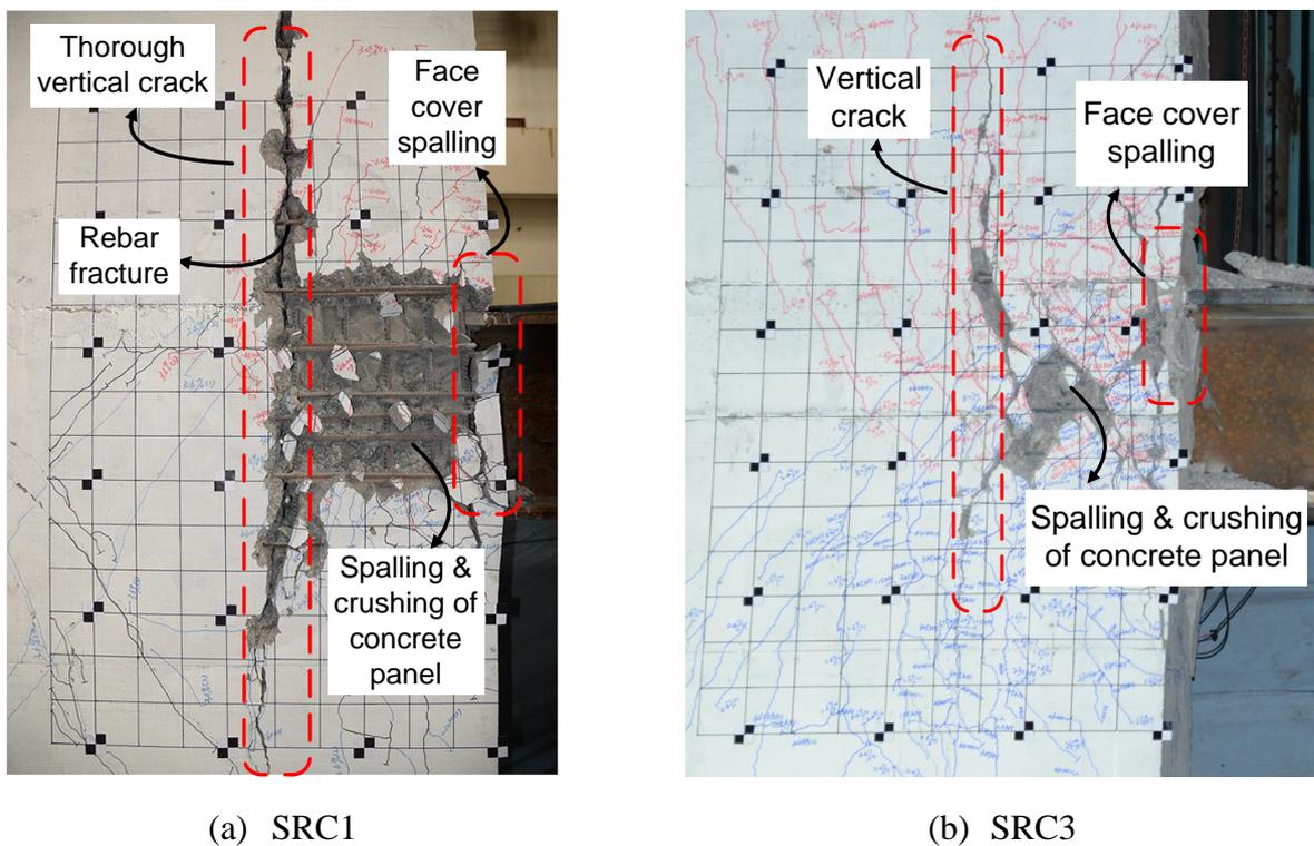
**Fig. 6.** Photographs of beam-to-wall joints of SRC1 and SRC3 at the end of testing.
