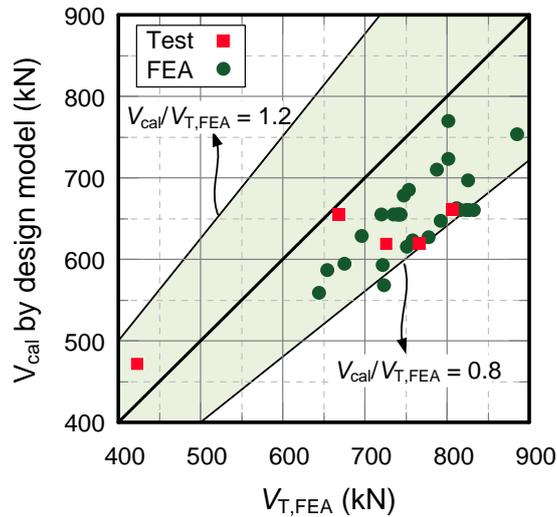
**Fig. 14.** Comparison between calculated nominal strength and experimental or FE results
