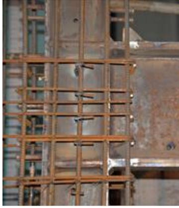
**Fig. 2.** Photograph of steel beam-to-SRC wall joint details.
