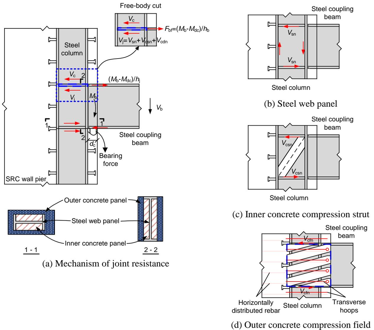
**Fig. 8.** Panel shear mechanism of steel beam-to-SRC wall joint
