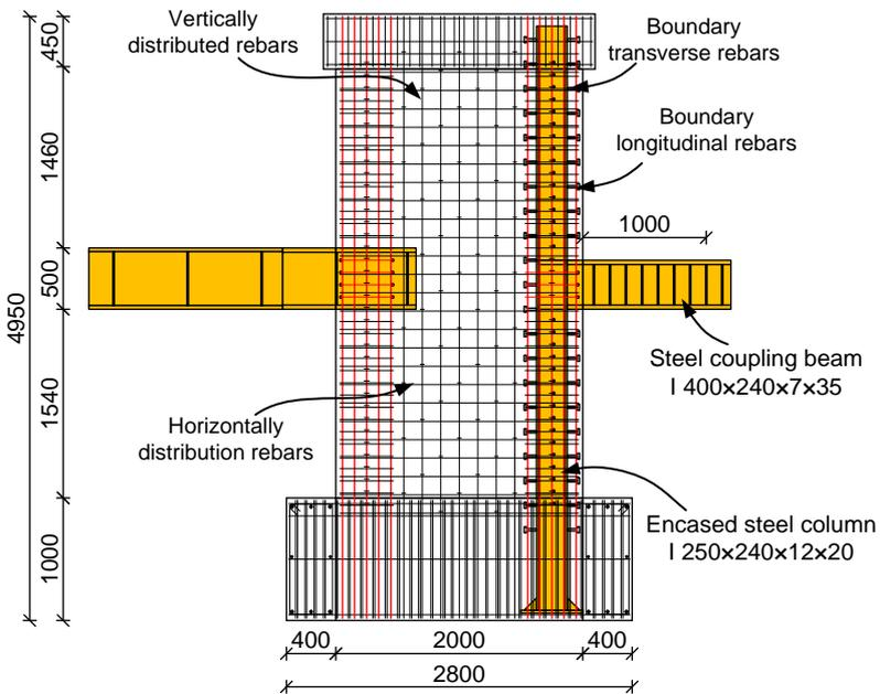
(c) Elevation drawing of steel reinforcement for SRC2
