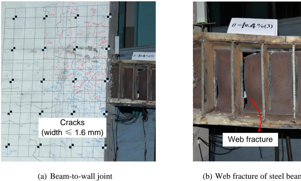
**Fig. 7.** Photographs of SRC2 at the end of testing.
