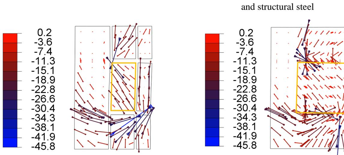
(c) Principal compressive stress of inner concrete (d) Principal compressive stress of outer concrete
