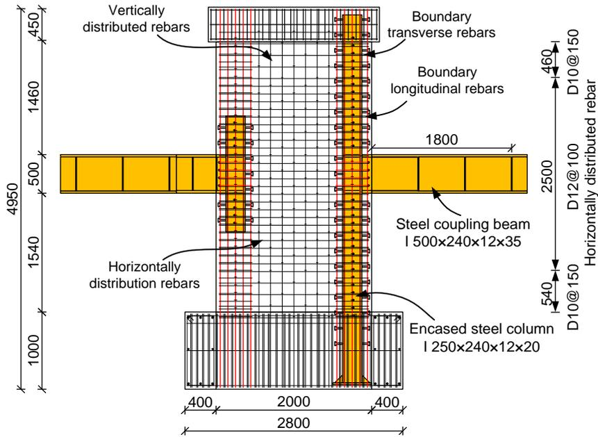
(d) Elevation drawing of steel reinforcement for SRC3
