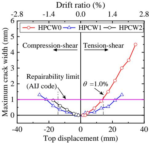
**Fig. 15.** Maximum crack width for all test walls.
