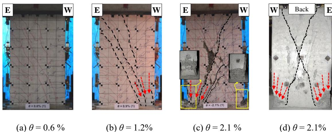
**Fig. 8.** Photographs of specimen HPCW2: (a) 0.6% lateral drift; (b) Peak lateral load; (b)
