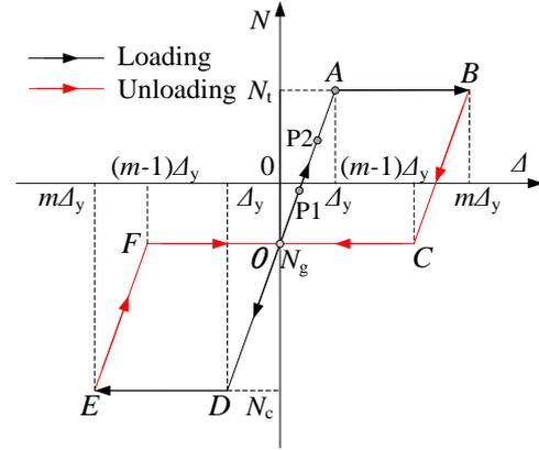
(b) Combined variable axial load and cyclic lateral loading
