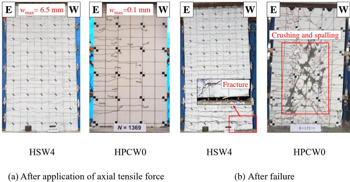
**Fig. 19.** Photographs of RC wall and PC wall specimens
