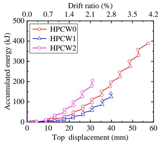
**Fig. 14.** Accumulated energy dissipation for wall specimens.
