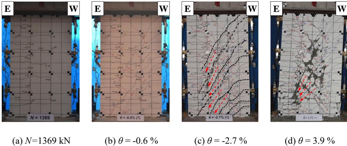
**Fig. 6.** Photographs of specimen HPCW0: (a) After applying axial tensile force; (b) 0.6% lateral drift; (c) Peak lateral load; (d) End of testing.
