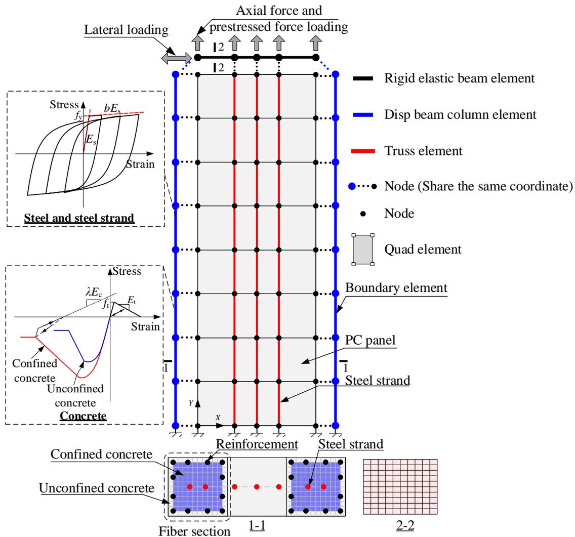
**Fig. 20.** Numerical model of PC wall.
