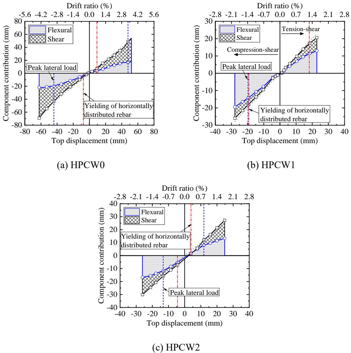
**Fig. 17.** Deformation components for all test walls.
