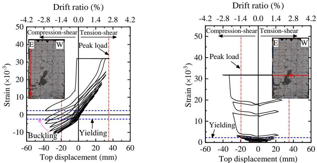
(a) Boundary longitudinal reinforcement      (b) Horizontally distributed reinforcement
