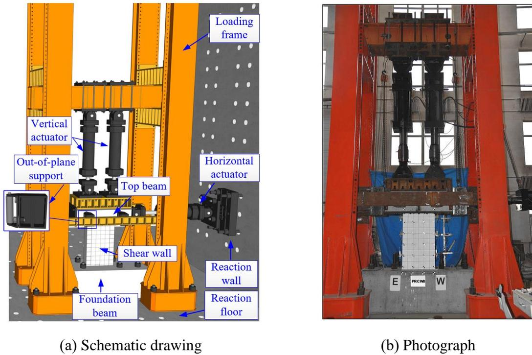
**Fig. 3.** Test setup.
