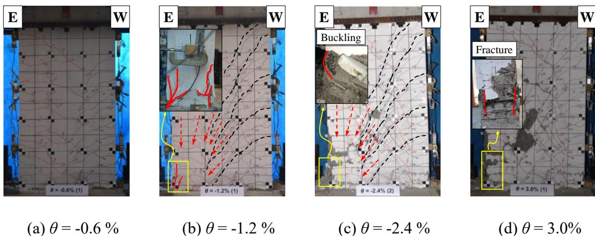
**Fig. 10.** Photographs of specimen HPCW1: (a) 0.6% lateral drift; (b) Peak lateral load in the negative loading; (c) Buckling of reinforcement; (d) Fracture of boundary reinforcement.
