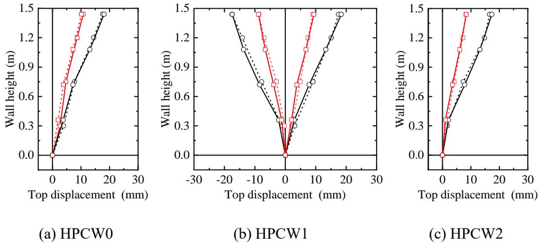
**Fig. 22.** Comparison of the lateral displacement response for all test walls.
