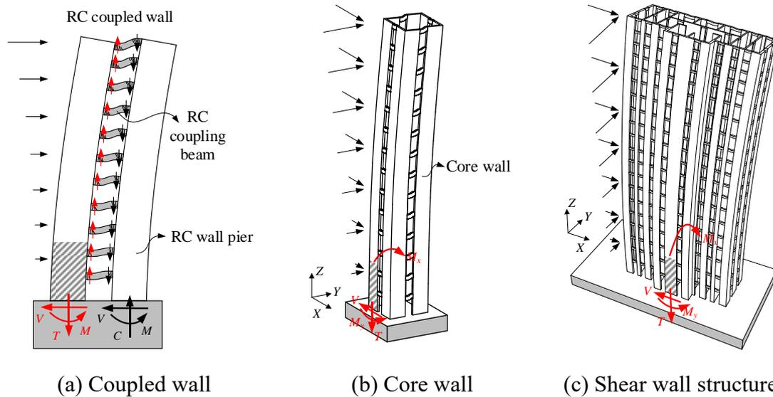
**Fig. 1.** RC walls undergoing combined axial tension, bending moment and shear force.
