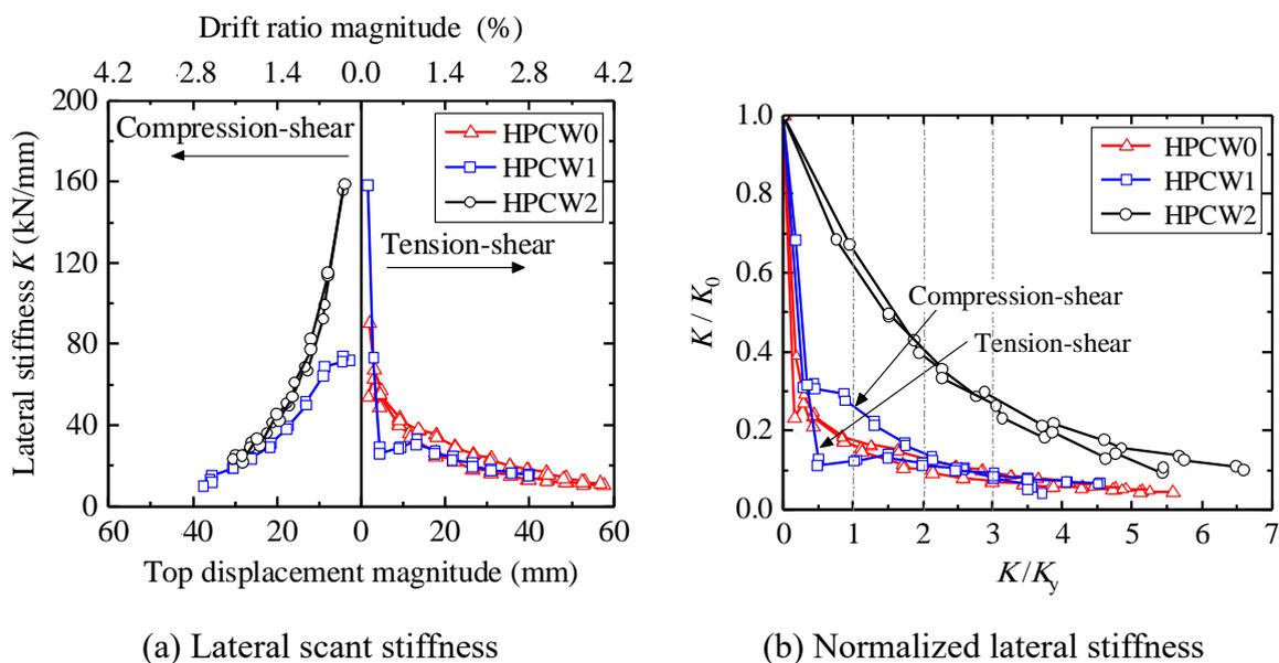
**Fig. 13.** Lateral secant stiffness degradation for all test walls.
