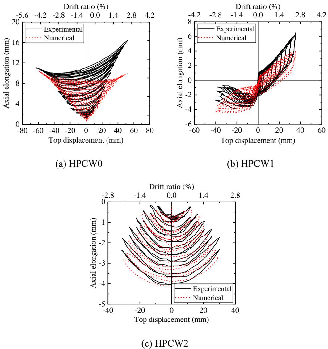
**Fig. 23.** Comparison of the axial deformation for all test walls.
