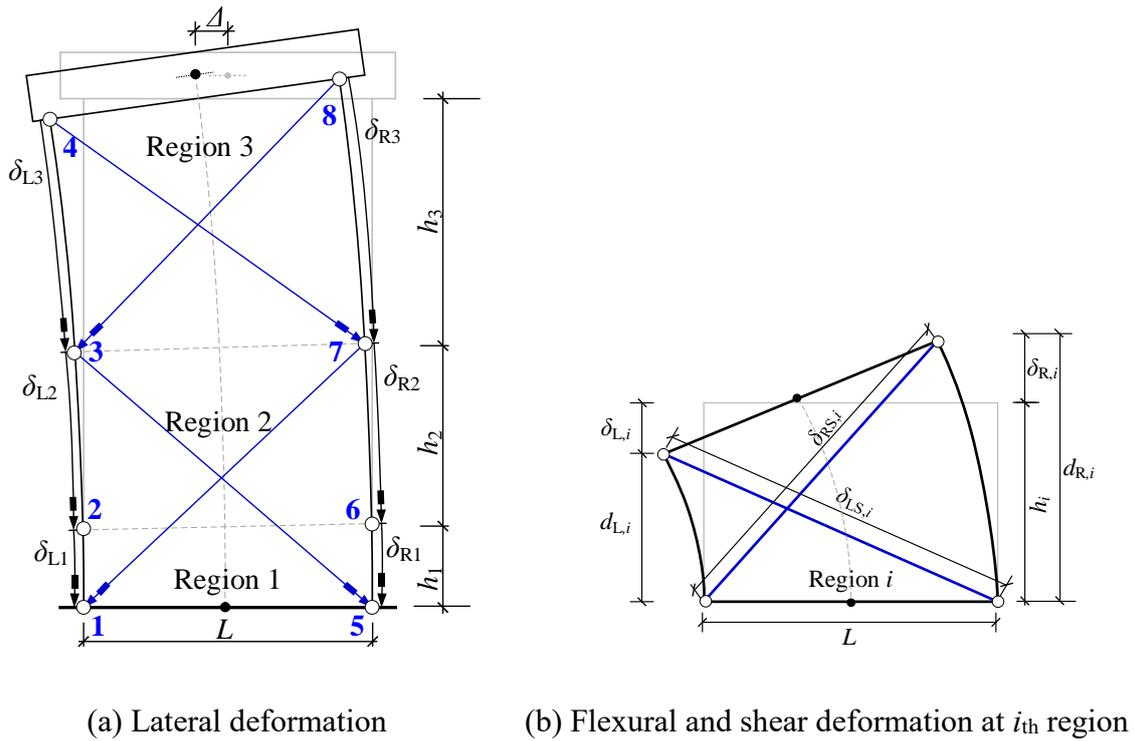
Fig.16 Calculation of flexural and shear deformations
