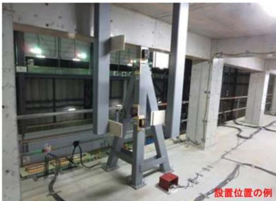
(a) Displacement transducer arrangement
